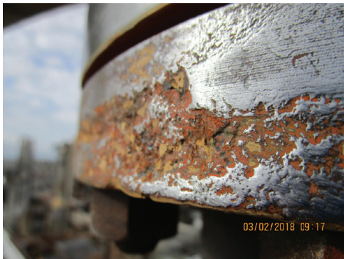
Figure 2. Rough Flange Surface
