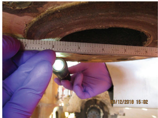
Figure 1. Visual Inspection Using a Straight Edge
